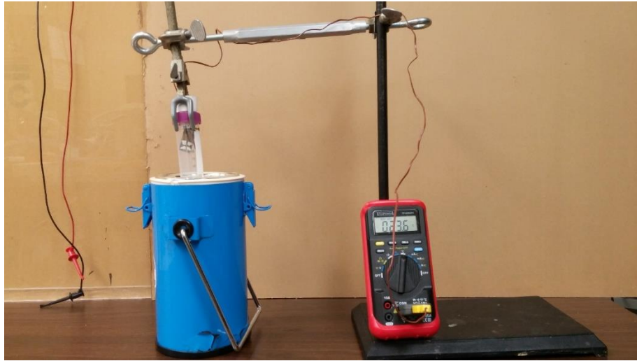
Figure 5.6: Low temperature measurement setup. Chemical mixture is prepared in the blue flask on the left.
