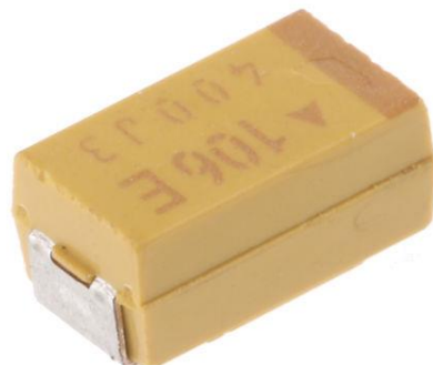
Figure 2.5: Finished surface-mount Tantalum capacitor [14].
