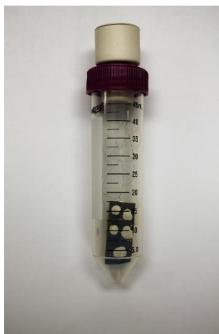
Figure 5.4: Test tube used for high and low temperature measurements. White rubber stopper through the cap is used to maintain the temperature inside the tube.
