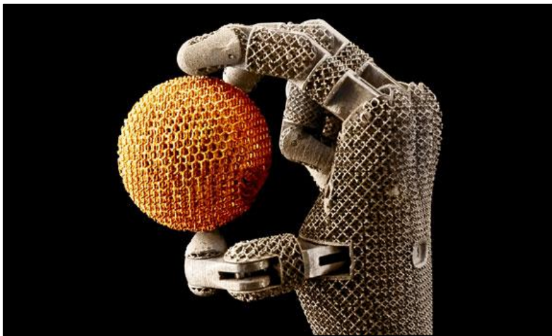
Figure 3: Parts manufactured from metal-laser sintering: handheld ball built bottom-up [4].
