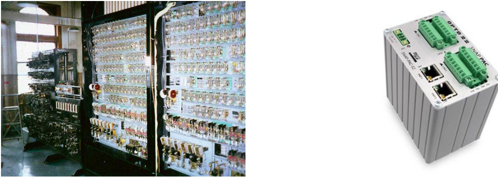
Figure 2.1: Left: Electrical Relay Bank, and Right: PAC with Ethernet and Serial Ports [wiki03] [wiki06]
