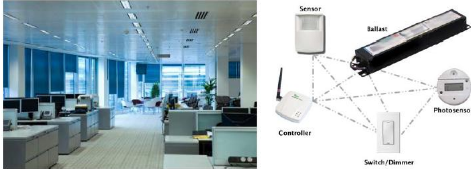
Figure 2.5: Left: Connected Real Estate with Automated Lighting, and Right: Lighting System Interconnection Diagram [dain01]
