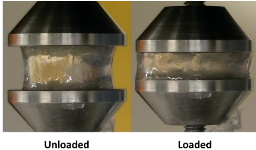
Figure 3.13: Unconfined compression mechanical Test of 3% Gelatin-1% Agarose at 40% strain and 1/s strain rate.
