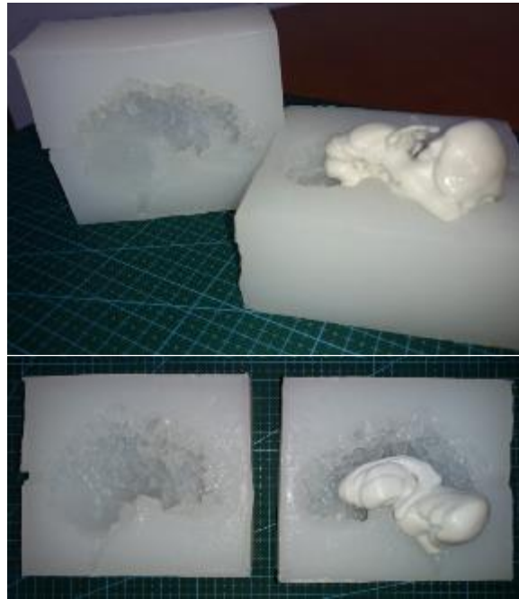
Figure 4.4: Brain cortex Negative Mold with 3D printed core brain positioned into place.
