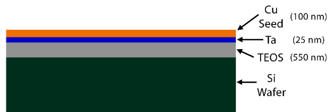
Figure 3.1: An illustration of SKW Associates Inc. blanket wafer cross-section prior to deposition.
