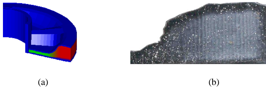
Fig. 1.1 Heterogeneous flywheel: a) representation, and b) cross sectional view of a fabricated heterogeneous flywheel made of 320 Stainless Steel and Copper Coated Nickel [Morvan2001].
