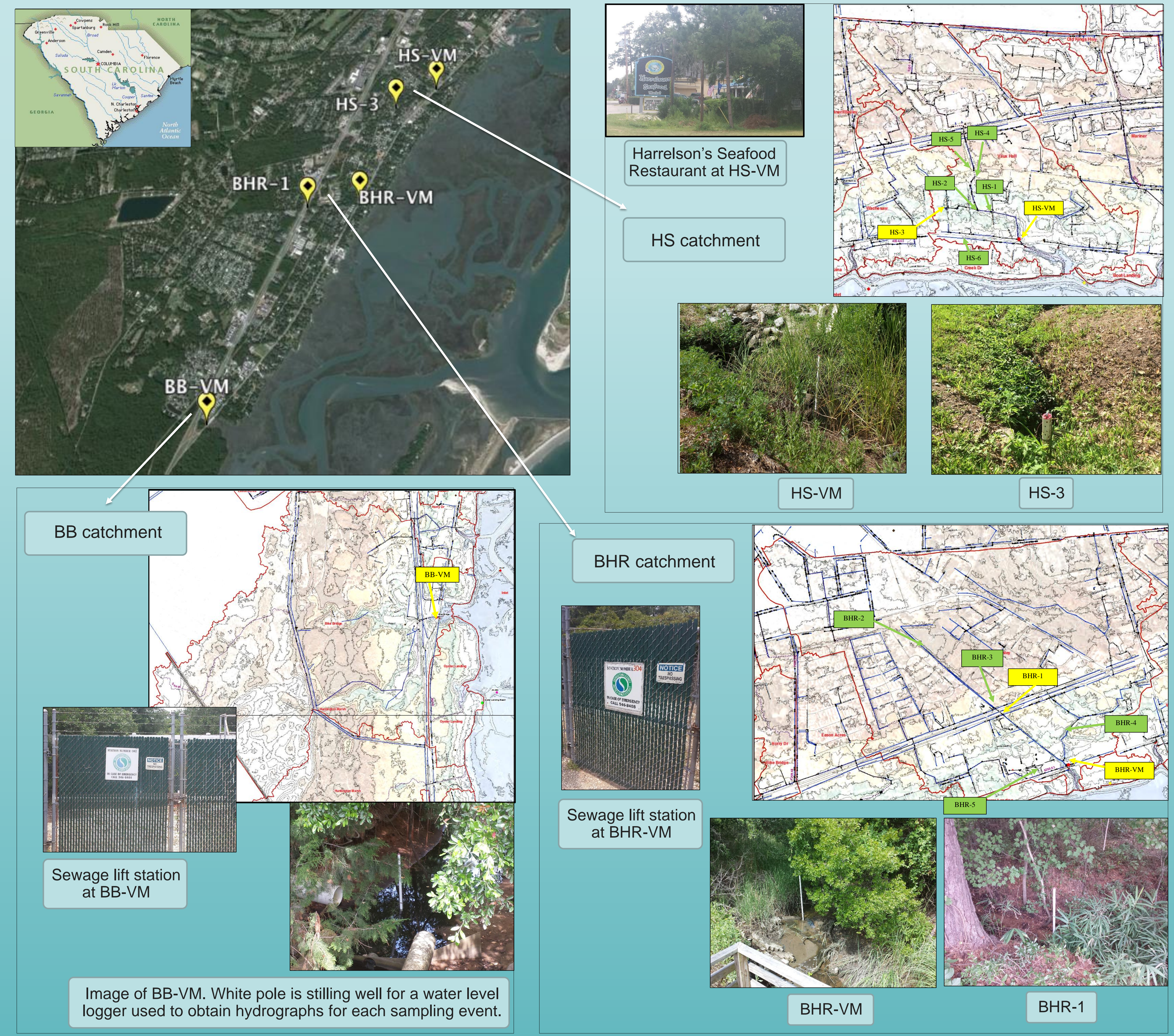
Figure 1: Map of Murrells Inlet with sampling sites with maps and photographs of each of the catchments. Phase I sites are in yellow. Potential Phase II sites are in green. Red lines are subwatershed boundaries. Blue lines are stormwater infrastructure.
