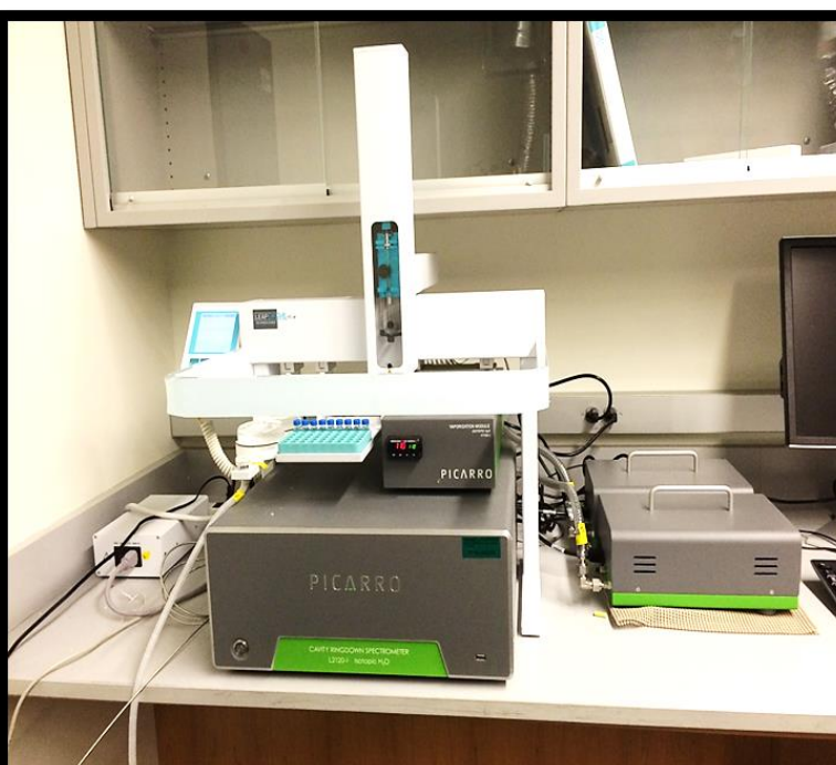
Figure 13. The analysis of stable water isotopes will be conducted through the use of a cavity ring-down spectroscopy liquid and vapor isotopic measurement analyzer (Picarro L2120-L, pictured).
