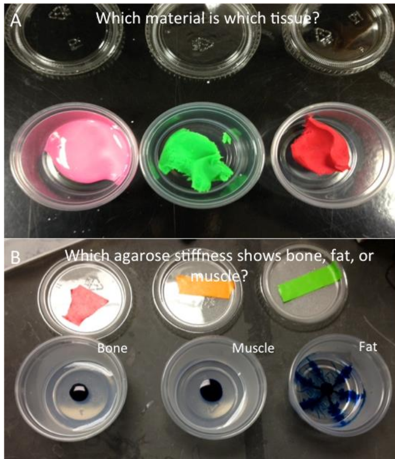
Figure 8.2: (A) Different materials with varying stiffness to represent muscle, fat, and bone tissues (B) The group activity where students determine the rate of movement of the dye solution in various agarose stiff gels
