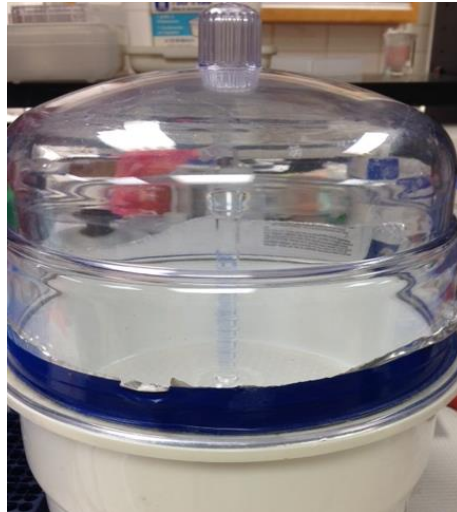
Figure 3.3: Experimental set-up to assess porosity in chronOS strip scaffolds with and without fibers
