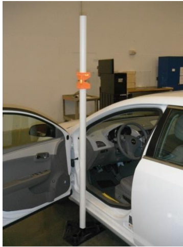
Figure 91. Vertical post rule to capture vertical position of eye-level, steering wheel height, and H-point height.
