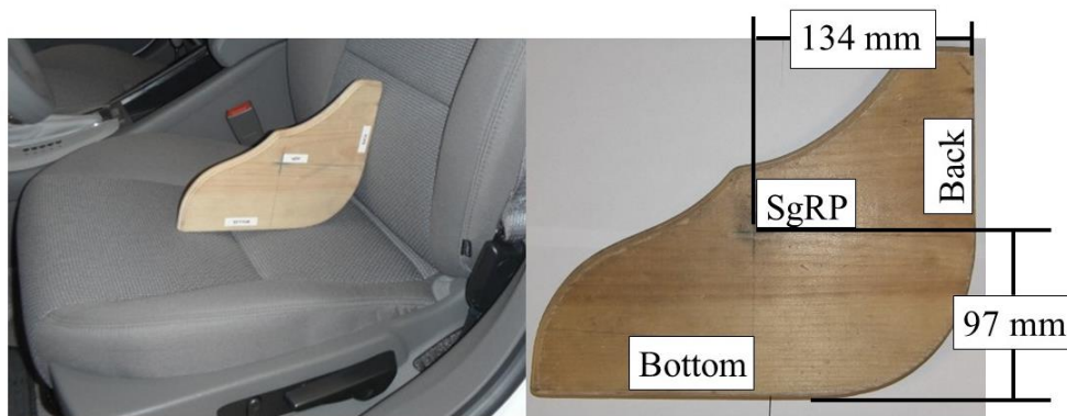
Figure 90. H-point jig to measure the location of the H-point. H-point Jig located in a vehicle seat (left) and laid flat (right).
