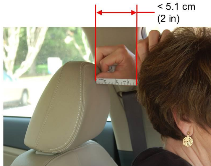
Figure 19. Horizontal distance from the back of the head to the front of the head restraint.
