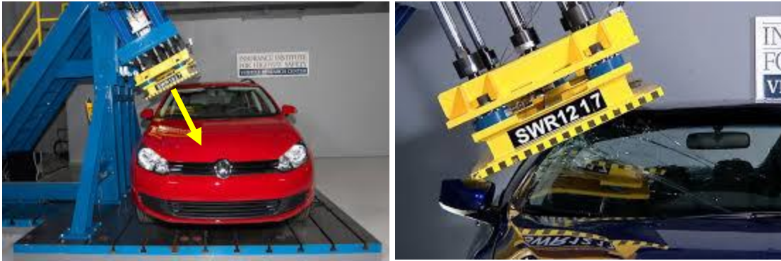
Figure 17. IIHS Roof Crush Test (Insurance Institute for Highway Safety, 2013d).
