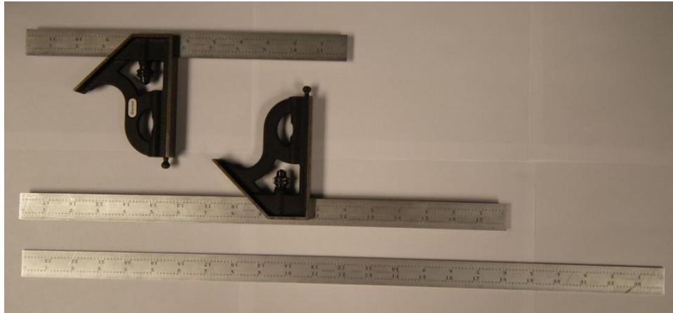
Figure 84. 12 and 18 inch combination square with a 24-inch combination blade.
