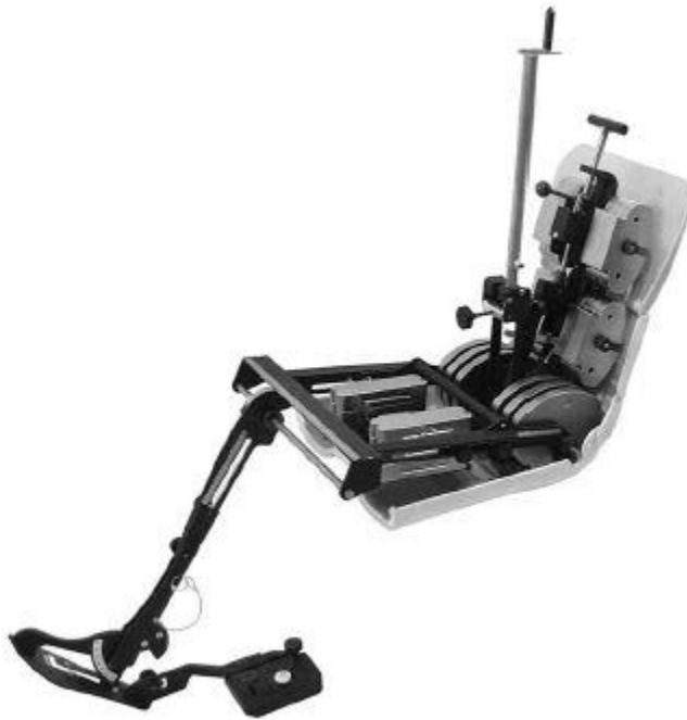
Figure 12. SAE J4002 H-point machine II (SAE International, 2010a).
