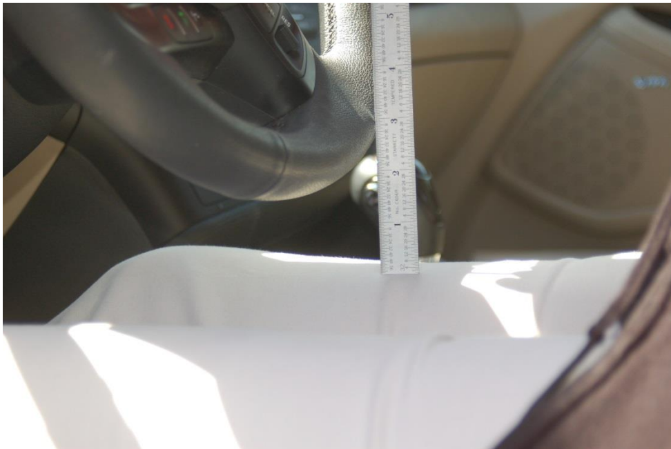
Figure 18. Measurement of the space between the upper thigh and the bottom of the steering wheel.
