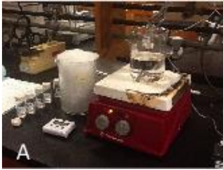
Figure 6.1. (A) Heat Stability Apparatus (B) Thermocouple measuring the temperature of the vial during heating.
