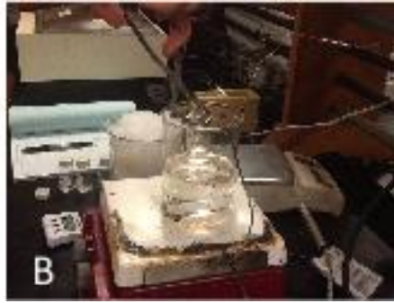
Figure 6.1. (A) Heat Stability Apparatus (B) Thermocouple measuring the temperature of the vial during heating.
