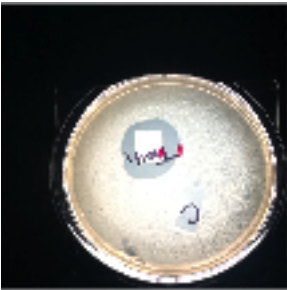
Figure 6.6. Plate overlay assay with film demonstrating antimicrobial activity
