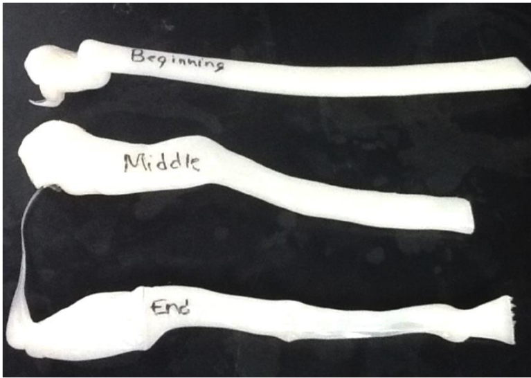
Figure 5.1. Extrudate from initial trials without the coat hanger die.
