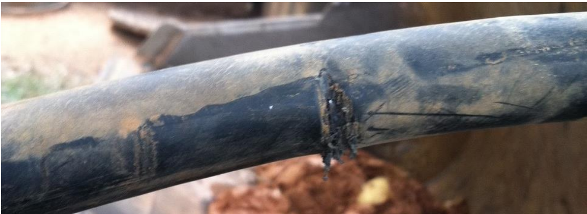
Figure 1.2: Another short circuited cable in Clemson
