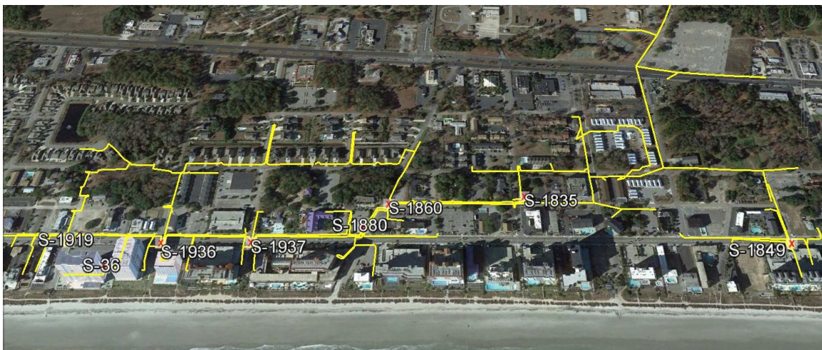
Figure 4.4: Google Earth image of distribution feeder on the coast of South Carolina
