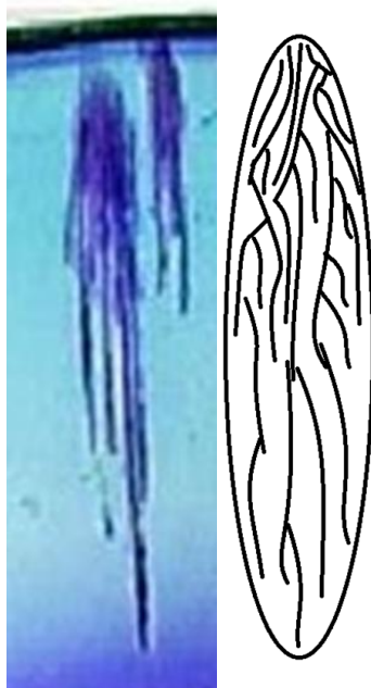
Figure 2.2: Single water tree and ellipsoid representation
