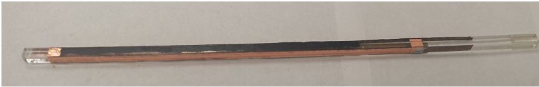
Figure 2.11: Actuator shaft with conductive ink painted on one side
