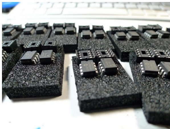
Figure 2.29: Conductive foam used to protect ICs
