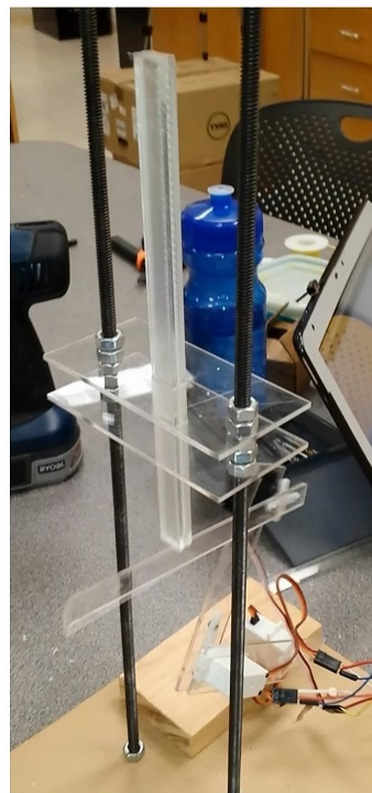
Figure 2.3: Prototype modified with extra servo motors
