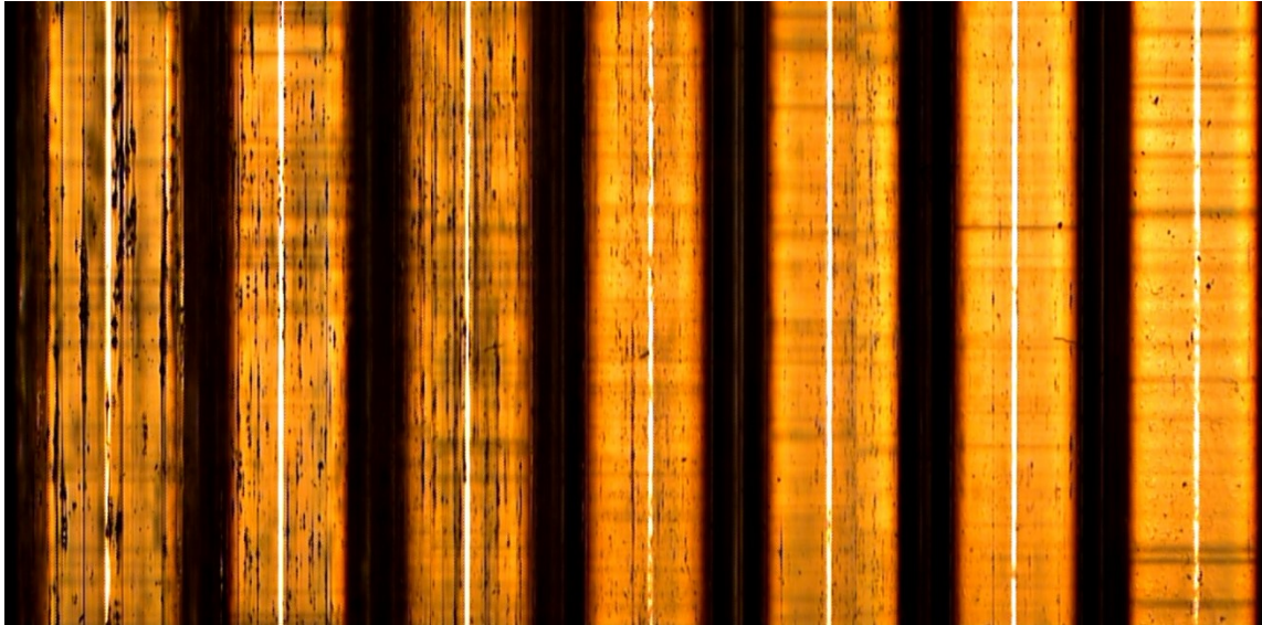
Figure 2.9: Shown is the lanthanum canes transition through draw. The canes crystallization decreased as the draw progressed (moving from left to right). This was largely due to the faster speed and higher temperature of the furnace.
