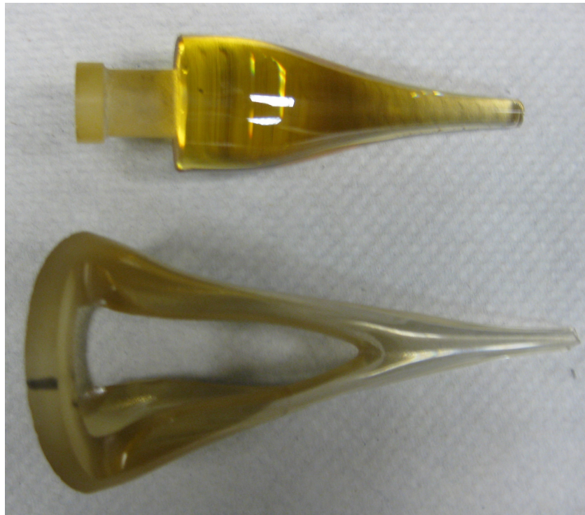
Figure 2.11: Neckdowns of the tellurite tube and rod.
