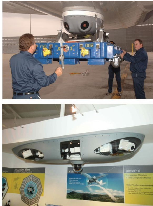
Figure 1.4: Infrared counter measure systems employed on commercial and military aircrafts. The depicted models are located on the bottom of the aircraft but IRCM can be located in more than one location on the aircraft including: top, front, and back so that they may cover all areas of attack [2].
