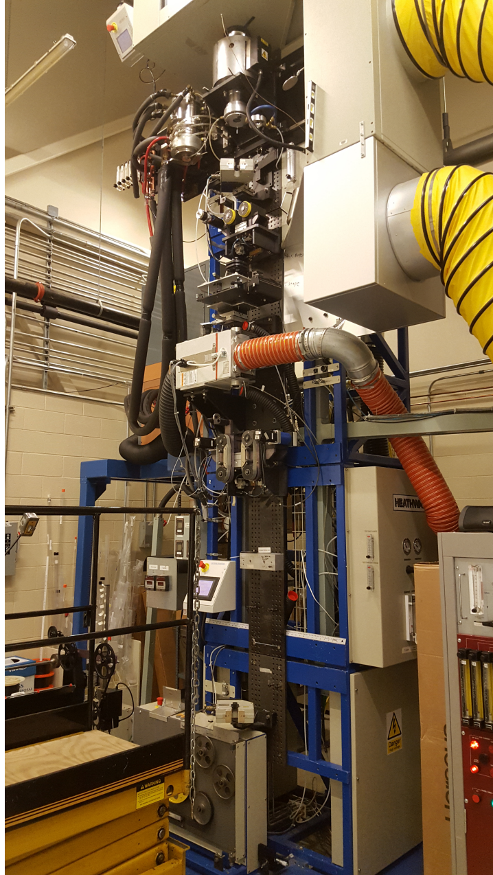
Figure 2.3: Clemson University draw tower with soft glass furnace in place.
