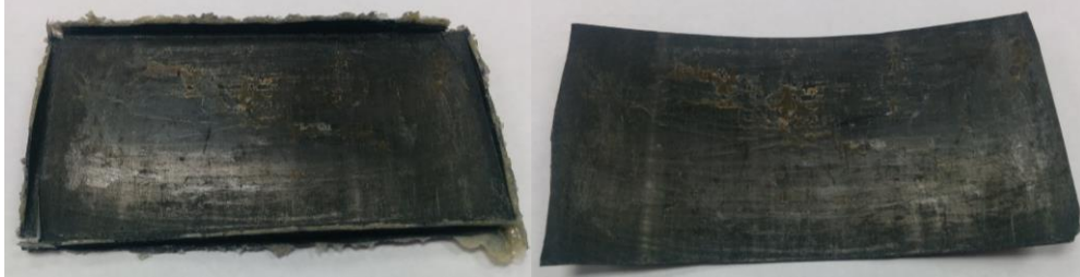
Figure 4.27: After curing (a) without trimming edges, (b) with trimmed edges
