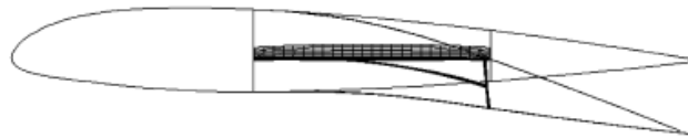
Figure 2.44: Lateral view of the stable shapes for camber change of airfoil section [23]
