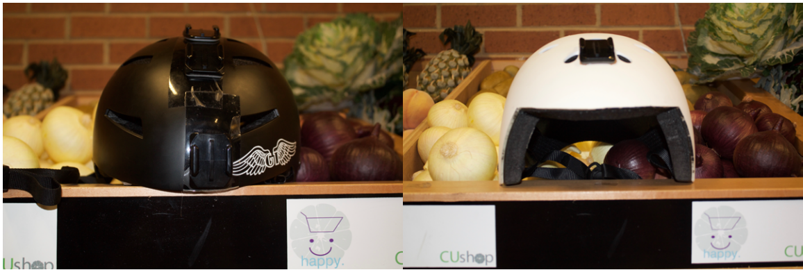
Figure 17: Prototype (left) compared to forehead cutout of the model (right)
