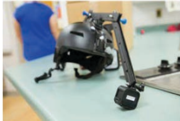
Figure 8: Prototype of facial expression analysis helmet
