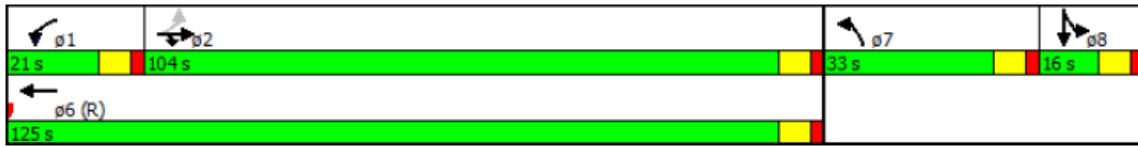
Figure 5-1: Manual Signal Operation Timings at US 76-US 123 Intersection
