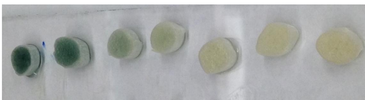
Figure 6.1.14. The test rolls under normal lab lighting on a sheet of clean glass with white paper for a background 5 min. after being dipped in varying concentrations of synthetic urine spiked with PPA. PPA concentrations go from high on the left ( 5 \times 10^{-4} M) to low on the right (no PPA).
