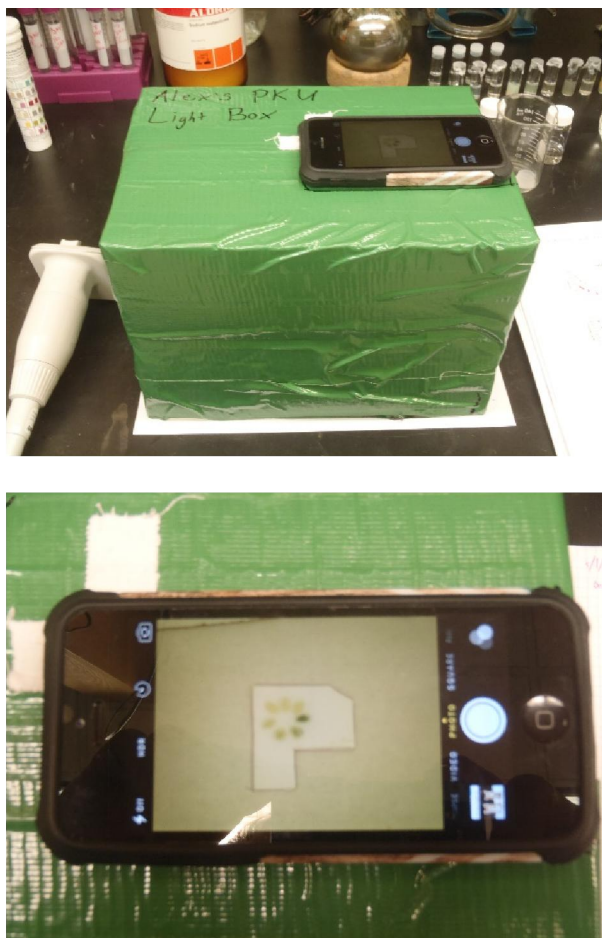
Figure 5.1. Light box in use. An oblique view (left) shows the box on a table with the iPhone in use on top. A top view (right) shows the screen of the phone viewing through the port in the top of the box to the illuminated the test samples below. The different colors of the test samples are due to their exposure to different concentrations of PPA.
