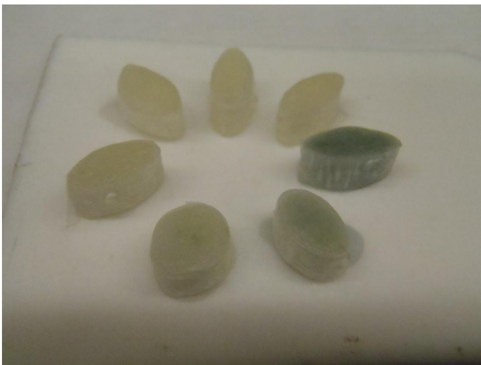
Figure 5.3 Seven test parafilm-wrapped paper-towel rolls shortly after being dipped in synthetic urine spiked with PPA. The rolls are arranged from highest PPA concentration to lowest in clockwise order starting with the sample in the far right middle of the circle.
