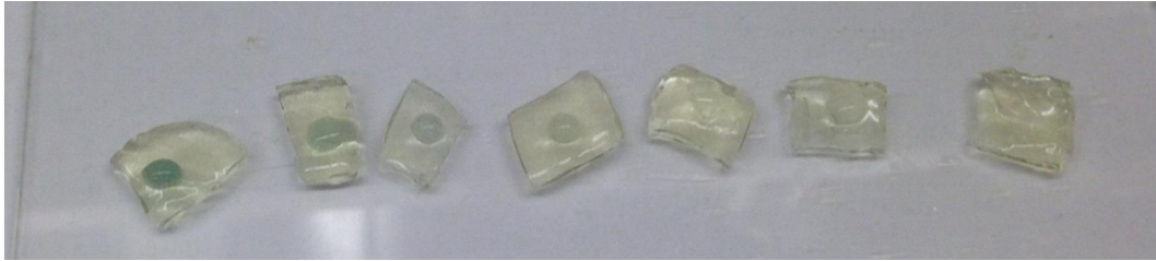
Figure 6.1.6. Fully hydrated hydrogel bandages with droplets of synthetic urine spiked with varying concentrations of PPA on their surface 5 min. after the PPA test solution was added. Concentration goes from high on the left to low on the right
