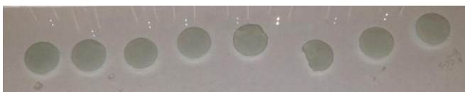
Figure 6.1.10. Anodisks pretreated with Phenistix 5 min. and then exposed to several different synthetic urine with varying concentration of PPA. PPA concentrations move from high on the left ( 5 \times 10^{-4} M) to low on the right (no PPA).
