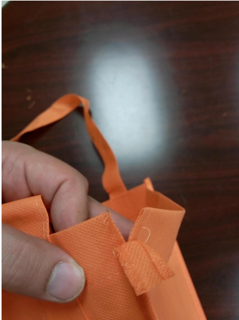
Fig. 3.12: Seam separation on a corner.
