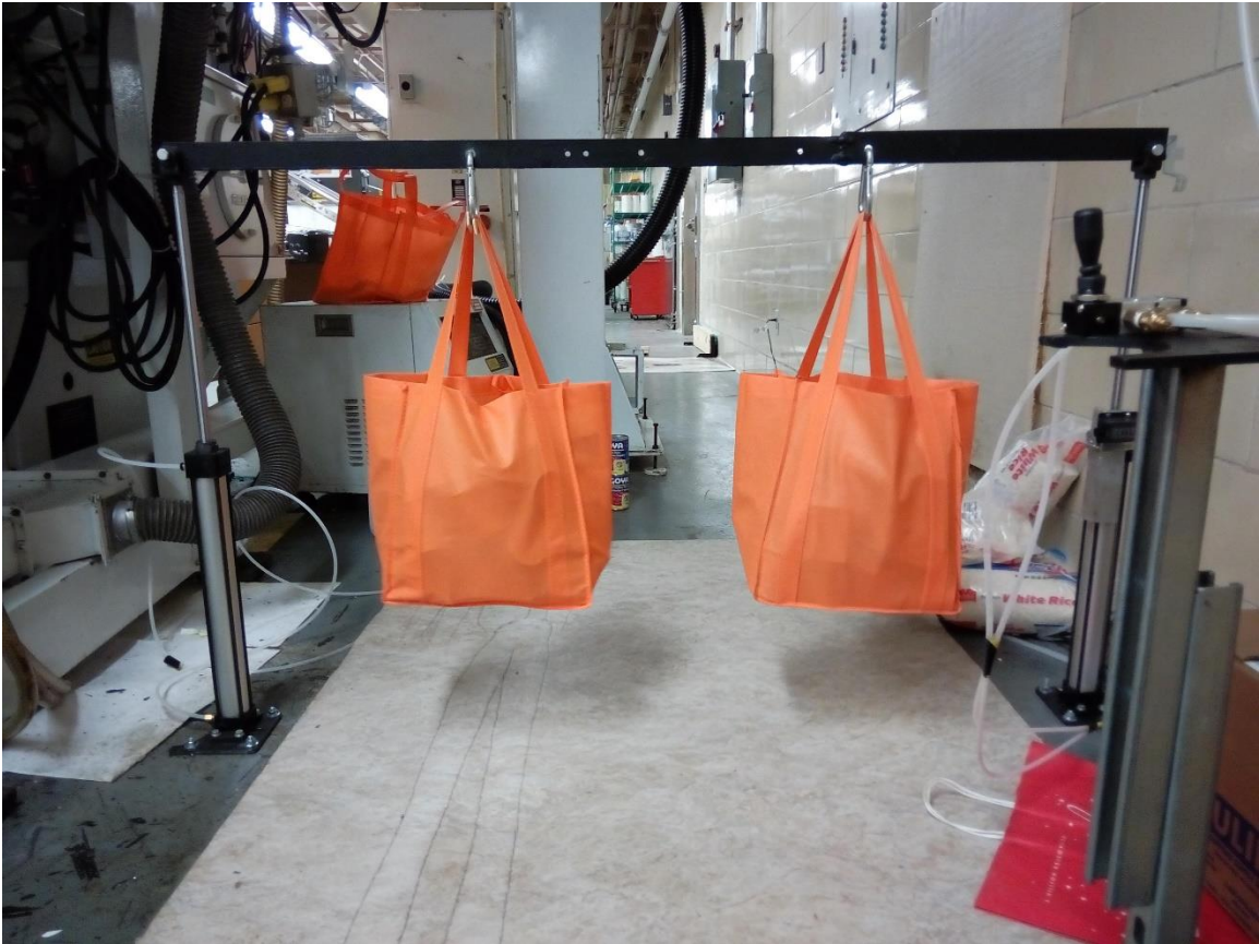
Figure 3.11: Apparatus with pneumatic cylinders extended
