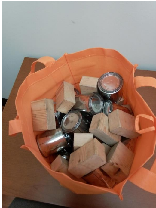
Figure 3.2: A NWPP bag loaded with wooden blocks, half-pint paint cans, and ball bearings (not visible).
