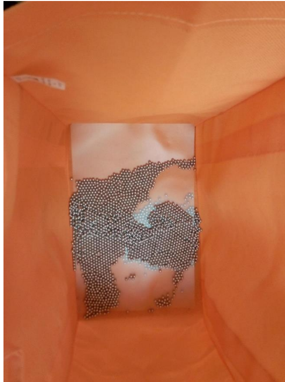
Figure 3.5: Ball bearings at the bottom of a NWPP bag, used as “granular material.”
