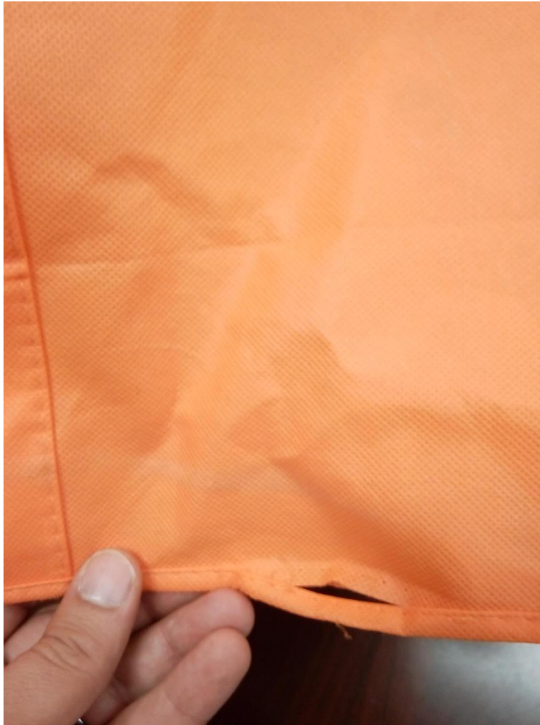
Figure 3.13: Seam separation on the bottom seam
