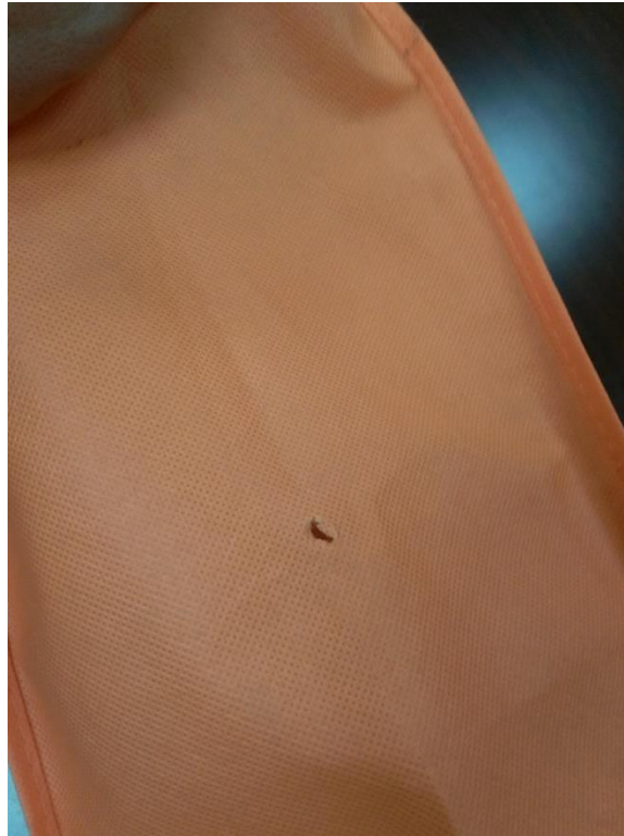
Figure 3.17: A hole. Note how the fabric does not fully “close.”
