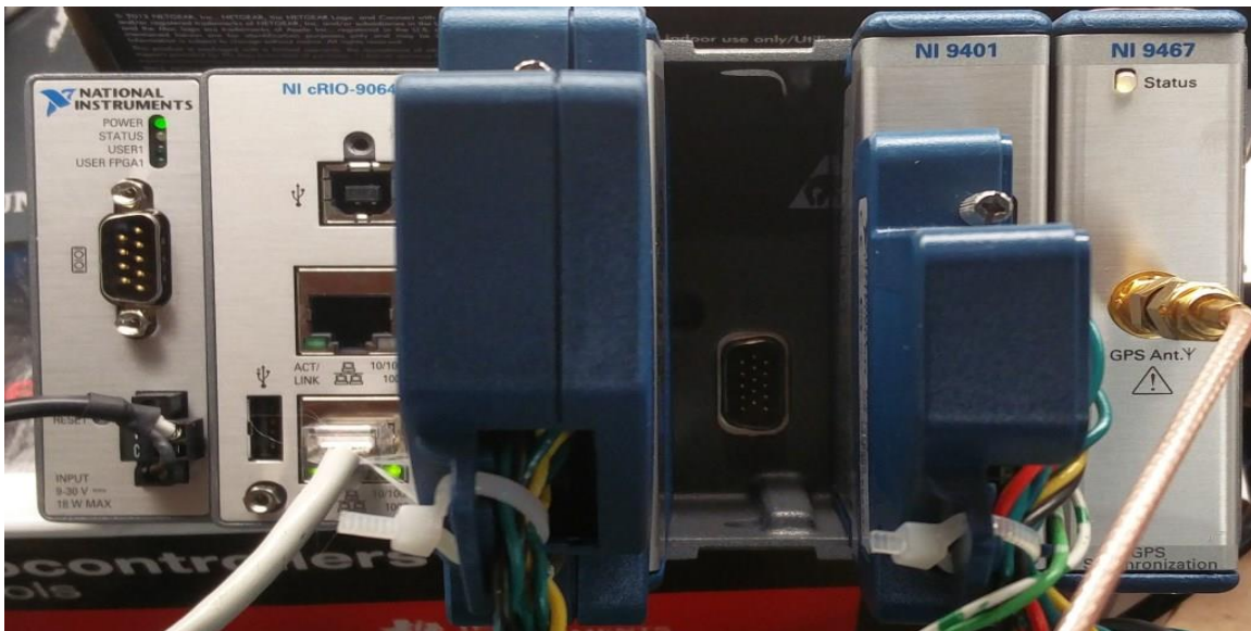
Figure B.2: NI CompactRIO 9064 used for Converter Side Controller prototype with C series modules NI 9220, NI 9401 and NI 9467
