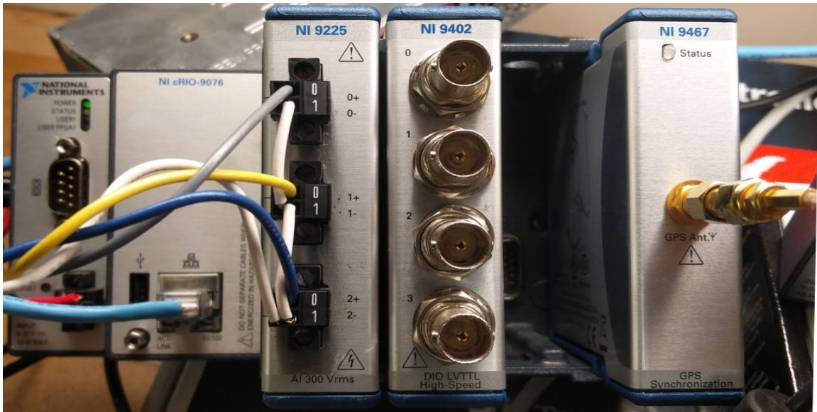
Figure B.1: NI CompactRIO 9076 used for Grid Side Controller prototype with C series modules NI 9225, NI 9402 and NI 9467
