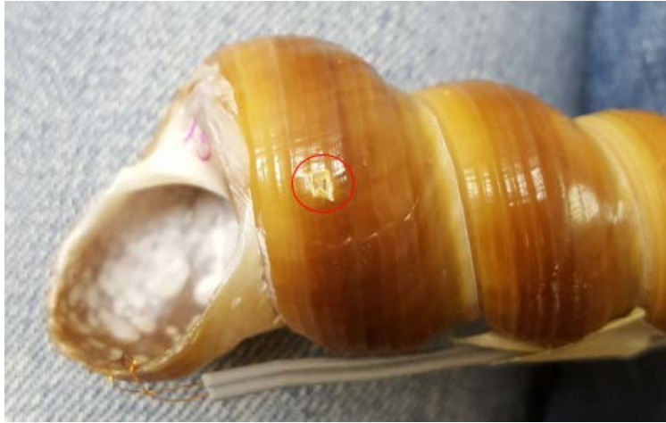
Figure 6.18: Local crushing (with no failure) observed in short-span shell after 35 lbs
