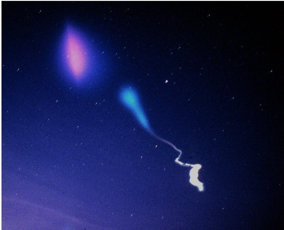
Figure 4.2: Sample image from the Guara campaign showing the partially ionized barium/strontium cloud (top) and the TMA trail (middle and lower). Figure from Kiene et al. (2015).
