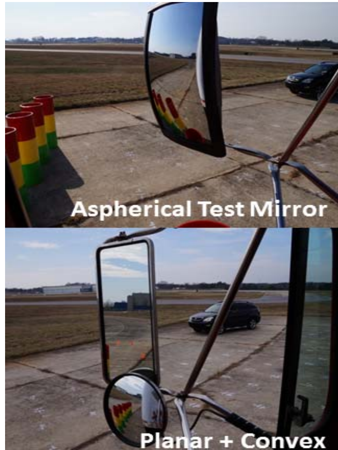
Figure 4.10 – Traditional Planar + Convex mirror as-installed (lower) & Prototype Aspherical mirror (upper)
