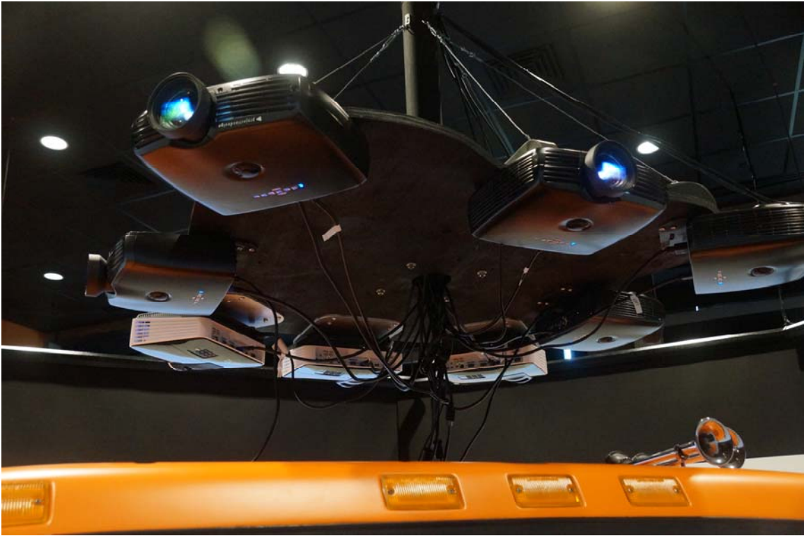
Figure 4.24 – Creative Car Laboratory Simulator existing five projectors
