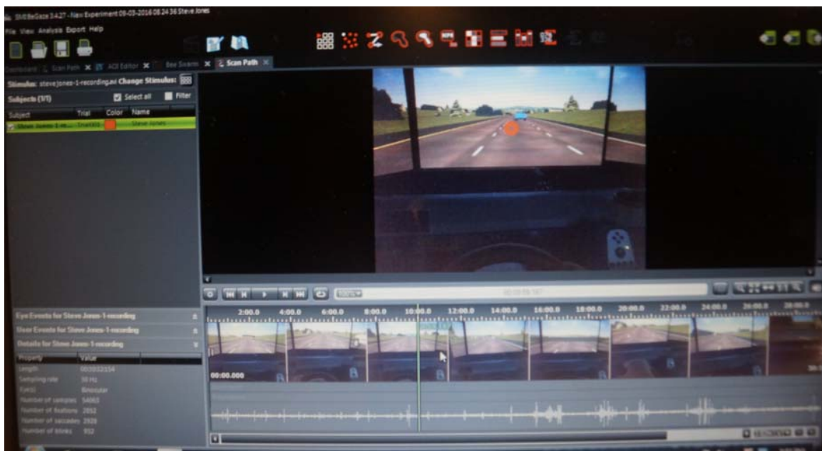
Figure 4.36 – BeGaze Software used for video-capture analysis of eye tracking data
