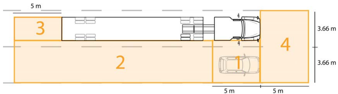
Figure 1.1 – Prioritized zones for driver vision improvement. The highest priority zone is indicated with numeral 1 [Reed, 74]
