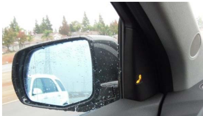
Figure 4.3 – Acura Blind-spot Alert System [Edmunds, 3]
