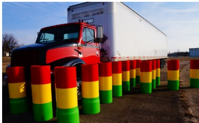
Figure 4.11 – Experimental test site, truck and targets used for performance of SAE J1750 target evaluation method.
