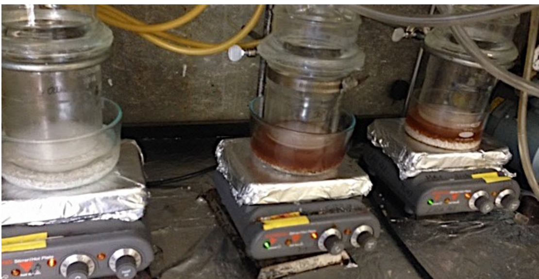
Figure 3.2: Setup of Reaction vessel used in synthesis of samples
