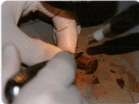
Photograph 8: Mechanical cleaning of nail with microtool
