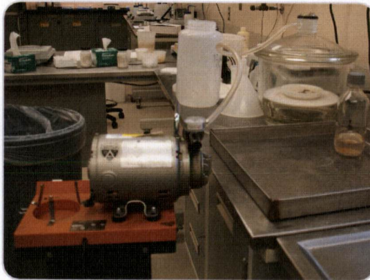
Photograph 4: Consolidation of key with acetone and resin in a vacuum
