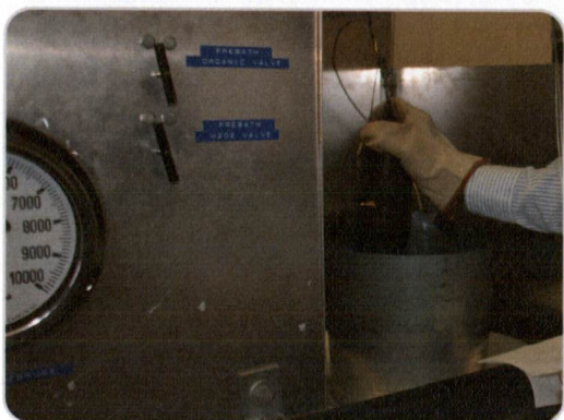
Photograph 4: Loading of subcritical chamber into heating element
