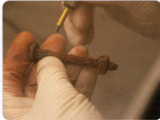
Photograph 9: Microabrasion of bolt
