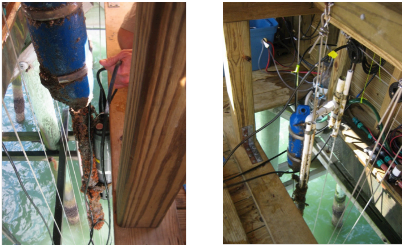
Figure 2. Pier monitoring station at the Second Ave. Pier showing ziplines and counterweighting. (a) Left photograph shows the surface sonde strapped to a PVC “sled” that slides vertically on two stainless-steel ziplines. The blue buoy is flotation that maintains the surface sonde ~1 m below the sea surface. (b) Right-hand photograph shows the zipline and PVC sled. To reduce biofouling, the sled is now fabricated from copper pipe. The blue box in the upper left corner houses the RAD-7 radon detector. Red hoses in the lower right-hand corner are part of a filter manifold that prevents particles from clogging the detector.
