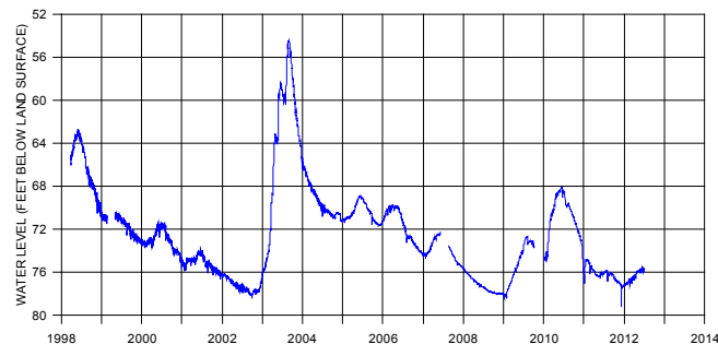
Figure 5. Daily average water levels for CRK-0074 (Crystalline Rock aquifer; open hole interval 99-265 ft).
