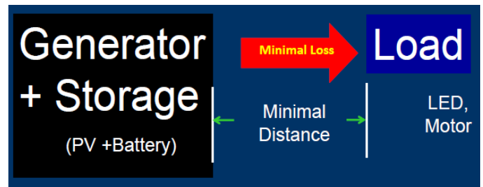
Fig. 5. Concept of local DC power with minimum distance between generation, storage and intelligent loads.
