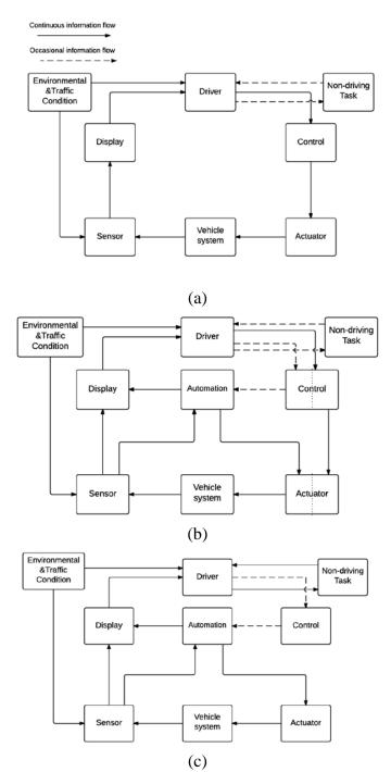
Figure 2. (a): Information flow at level 0 (within control loop); (b): Information flow at level 1 (partially out of the loop); (c): Information flow at level 2 and 3 (approximately
