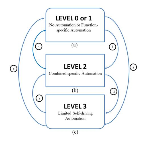
Figure 17. The transitions between each levels of automation (a) Level 0 or 1 automation; (b) Level 2 automation; (c) Level 3 automation
