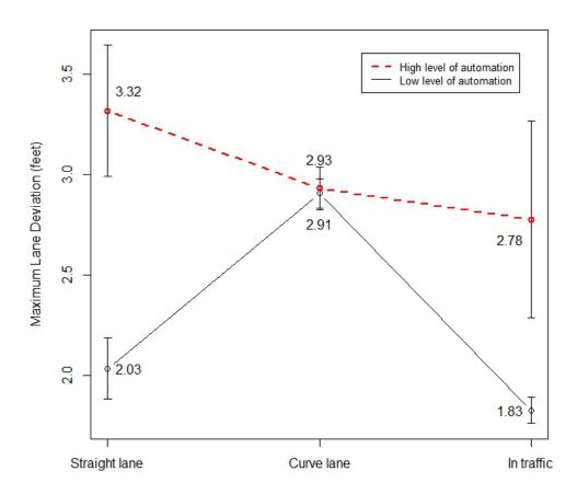
Figure 7. Maximum lane deviation (and standard error bars)
