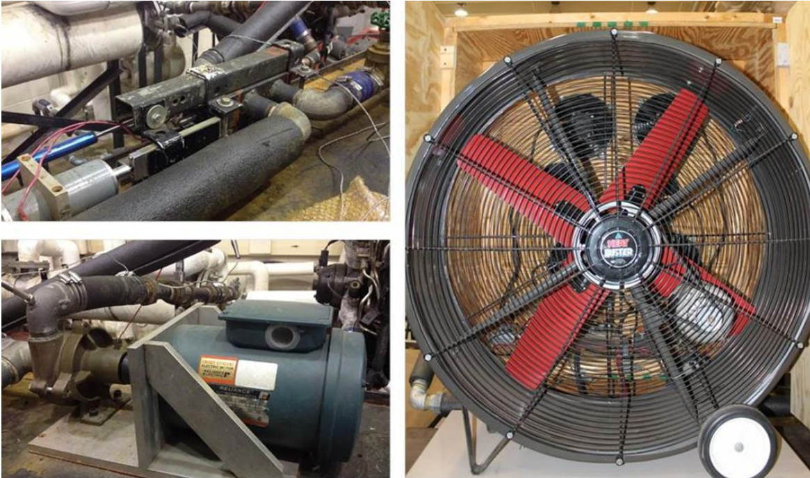
Figure 5.4: Picture of experimental test bench - smart valve, coolant pump, and radiator fans with ram air axial fan
