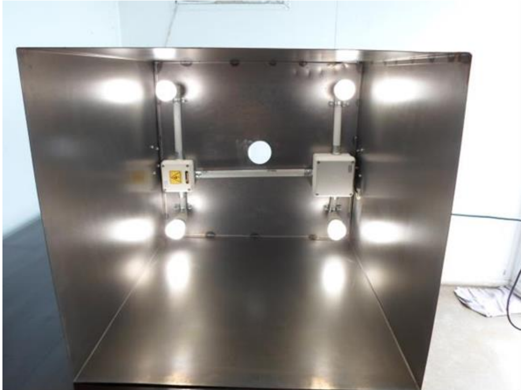
Figure 4.5: Light arrangement inside of the light box used to take digital photographs for assessment of disease intensity (DI t ) on the practice tee at Pilará GC, Pilar BA, Argentina.
