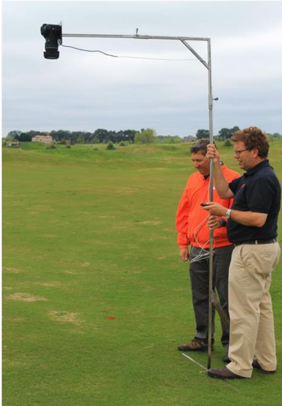
Figure 4.2: Digital photographs of entire sub subplot taken with a monopod for disease incidence assessment on the practice tee at Pilará GC, Pilar BA, Argentina.
