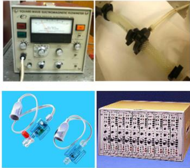
Figure 2.6: FM501 Electromagnetic flow meter (Upper left) and EP640 flow probe (Upper right); blood pressure transducers (lower left) and bridge amplifiers (lower right).
