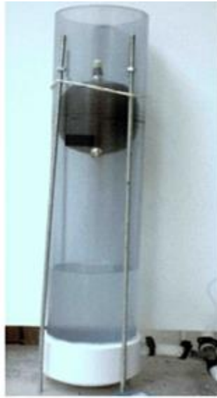
Figure 2.5: Photograph of an air chamber compliance element.
