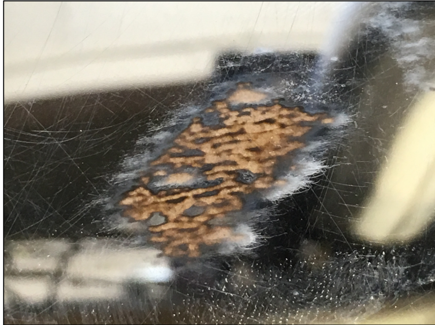
Figure 4.2: Damage on aluminum coated PE surface caused by friction and heat
