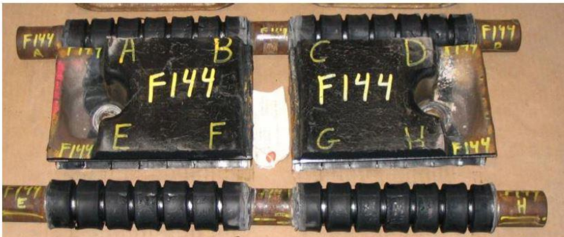
Figure 1.3 Embrittlement and Cracking of Backer Pad and Bushing Assembly [6]
