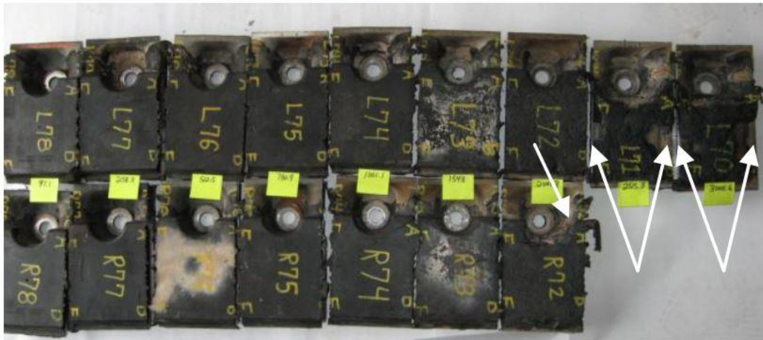
Figure 1.4 Progression of Chunking of a Backer Pad [6]
