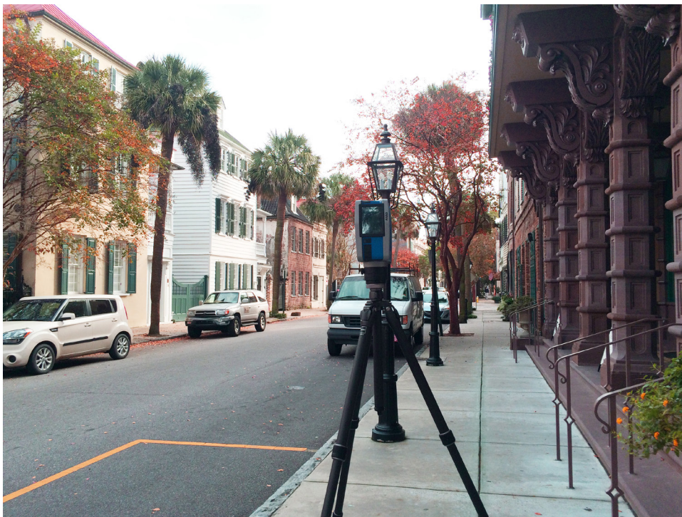
Figure 5.6 - Laser Scanning Data Accumulation on Trial Block.
