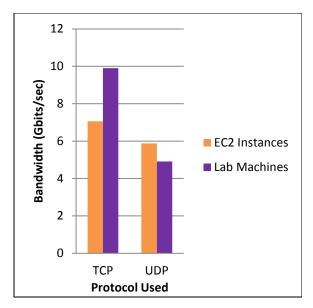
Figure 5.1: AWS HPC Cluster project EC2 Instances no Placement Groups or Enhanced Networking vs Lab Machines (MTU 9000)
