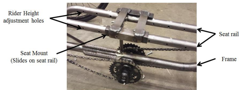
Figure 3. Seat rail, holes, and seat mount for seating system adjustments A.) Side view B.) Top view
