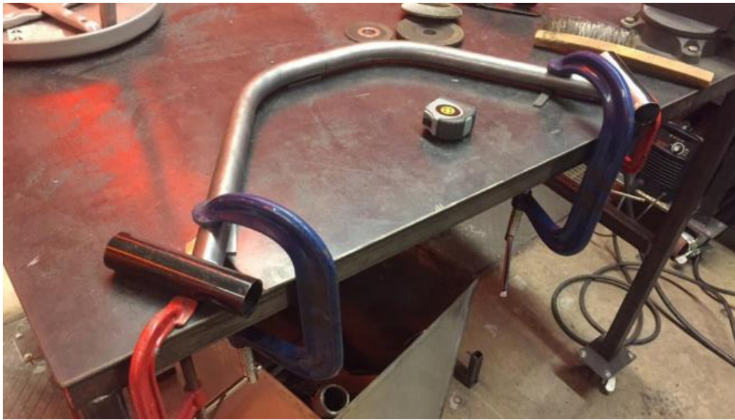
Figure 5.6 Jigging for steering arm and head tube connections
