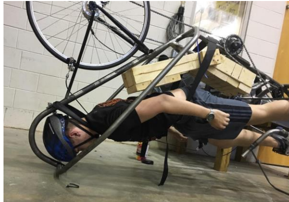
Figure 3.3 Rider harnessed in vehicle upside down
