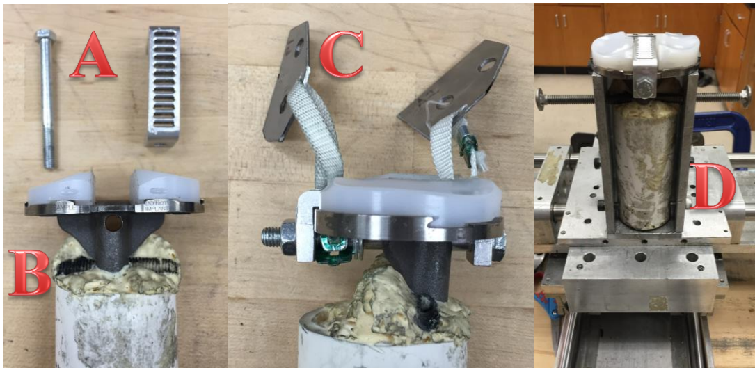
Figure 9.7 Tibia attachment fixture and assembly: tibial attachment (A), tibial baseplate (B), ligament attachment (C), and xy-table setup (D)
