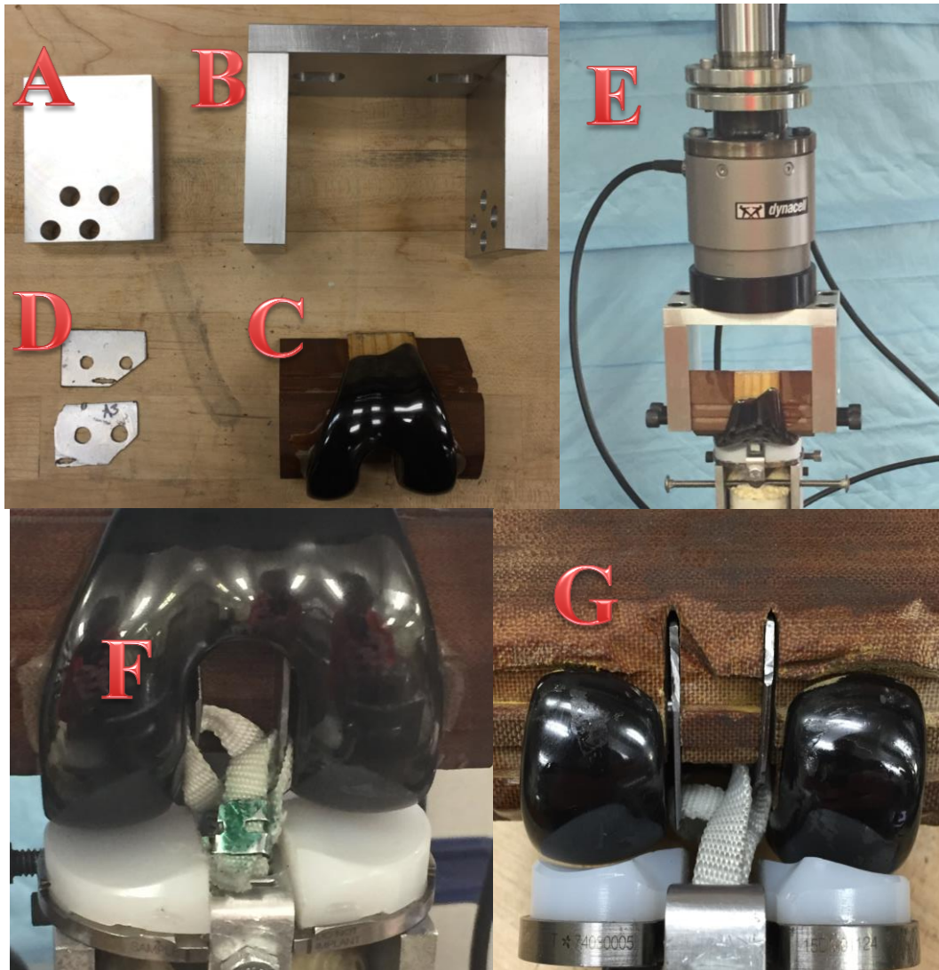
Figure 9.6 Femoral attachment fixture and assembly: side blocks (A), femoral attachment (B), femoral block (C), sliders (D), full assembly (E), and ligaments inserted (F and G)
