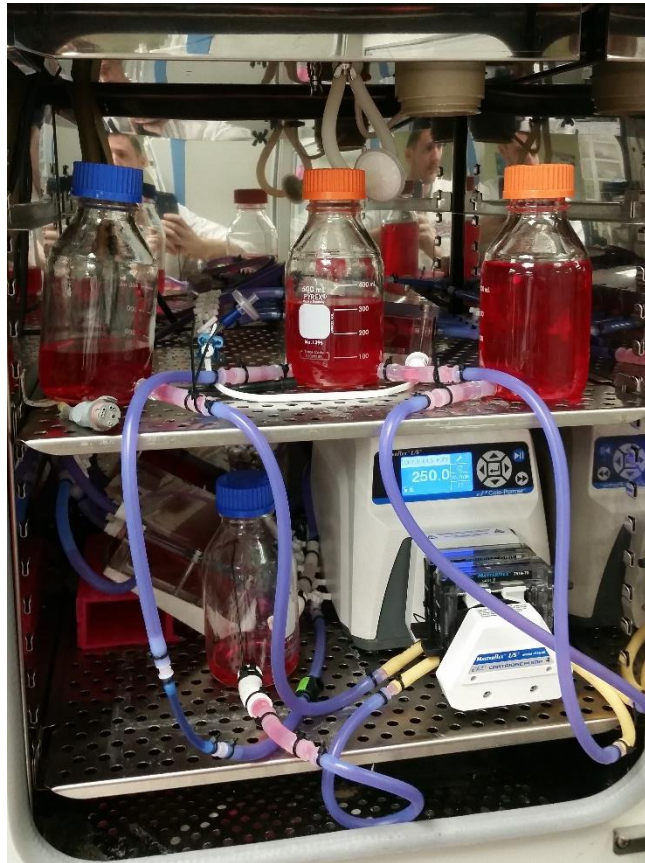
Figure 5.4: Normal and High Glucose Vascular Bioreactors in an Incubator Just Prior to Removal
