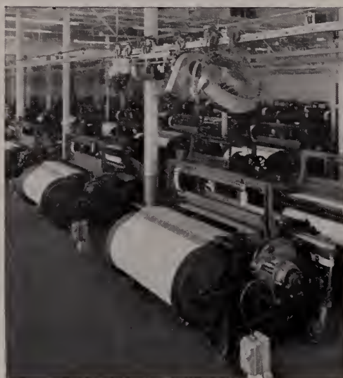
with automatic loom and ceiling cleaning 57% of manual cleaning is eliminated. Ceilings are blown-down once a month instead of every week.
