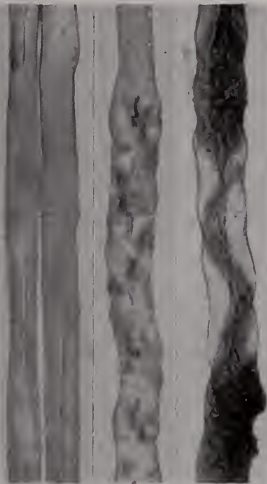
Figure 1. CONGO RED TEST: left, undamaged fibers; center, slight mechanical damage (note stained damaged spots); right, seriously mildewed fiber (upper and lower portion stained). (250 X).
