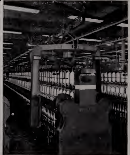
Underframe unit mounted on old cleaning system to complete cleaning operation.
