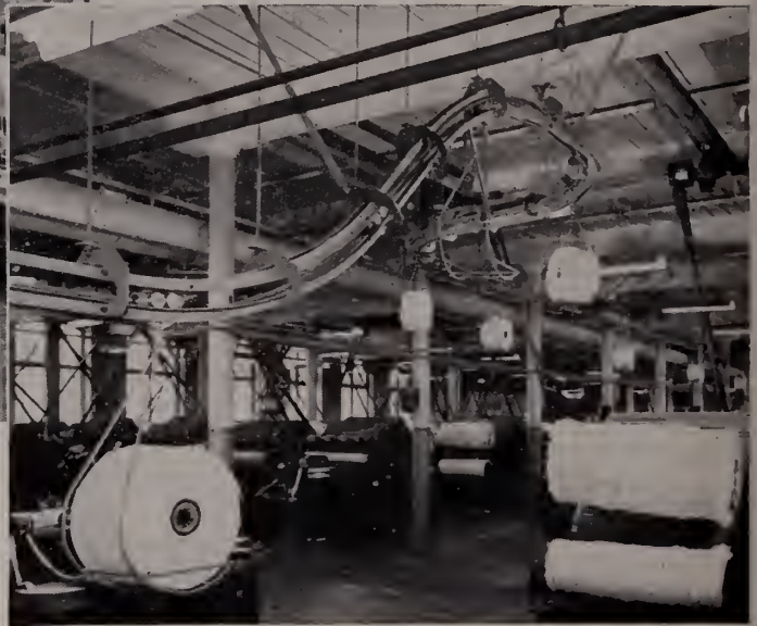
Complicated curves are no problem with Landahl Chainless Conveyor. The light track sections are easily fabricated into short radius turns in any direction.
