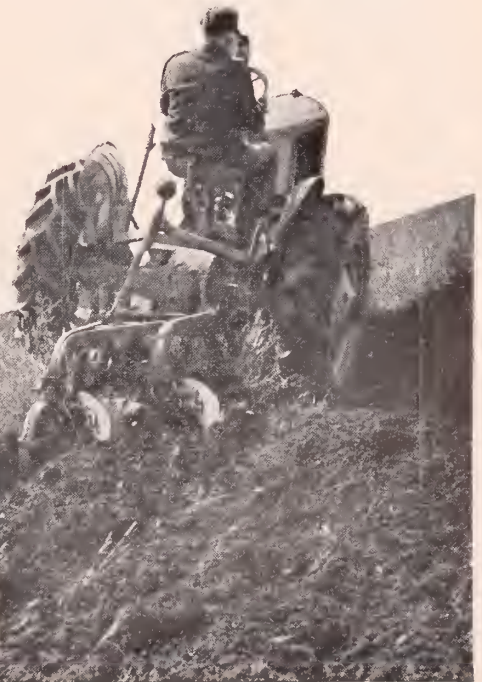
Case Model "VAC" tractor with 2-bottom rear-mounted plow.
