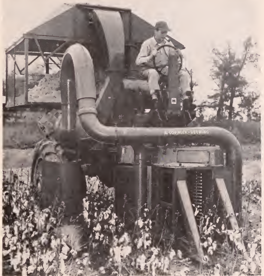
The author is shown above piloting one of the modern McCormick-Deering cotton pickers being used in the South.
