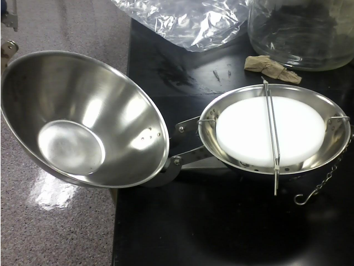
Figure 2.4: Inside of a PAS with PUF disk in wire carrier.
