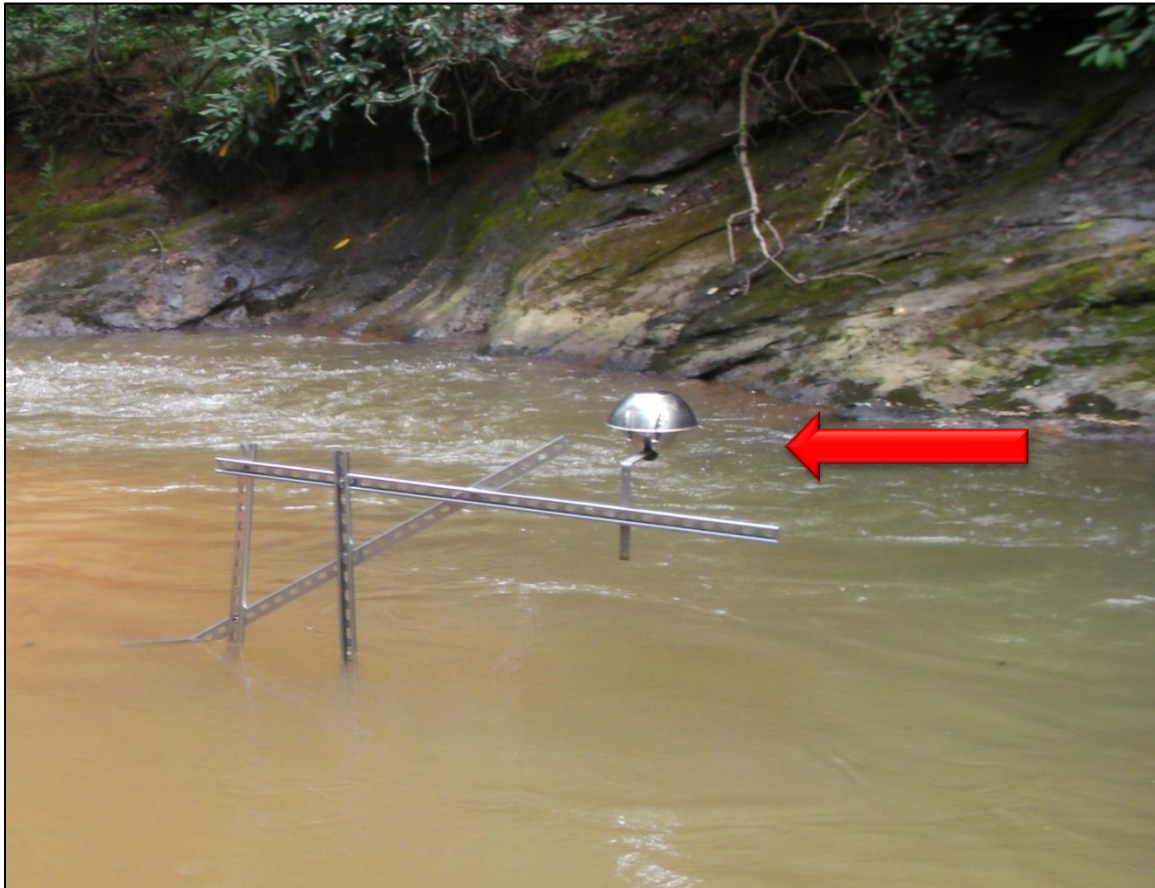
Figure A.2: PAS unit (S1) assembled and installed over Town Creek.
