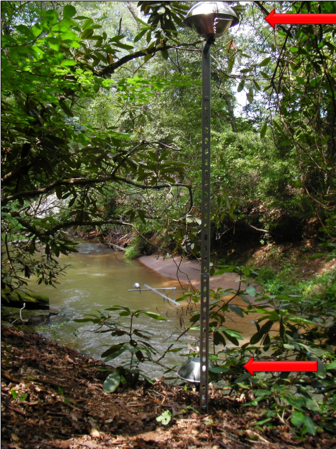
Figure A.1: Fully assembled and installed PAS units (S2 and S3).
