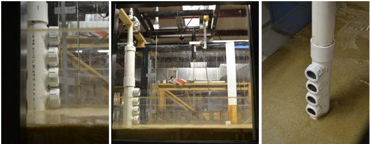
Figure 3.4 – Prototype VTP array installed in flume bed. VTPs 1-4 are shown (right/left) above the sand bed, housed in support pipe (middle) connected to the flume frame.
