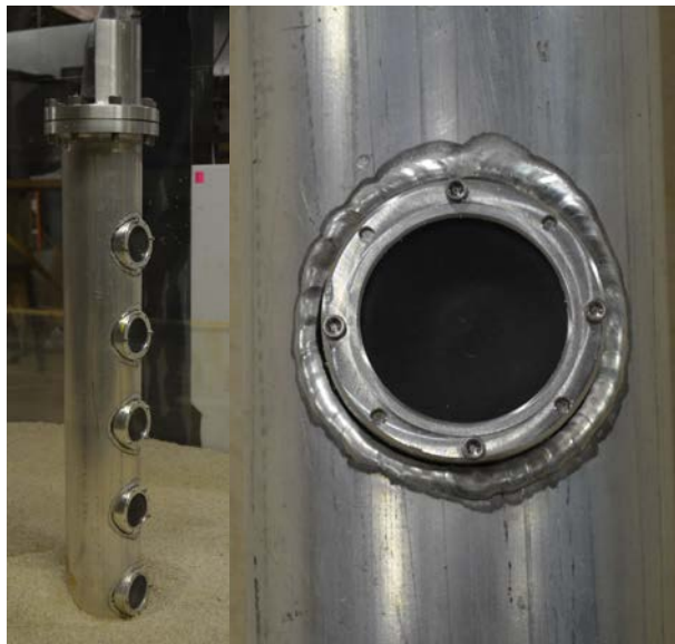
Figure 4.1 - VTP setup as installed in CHL flume for channel effects study.
