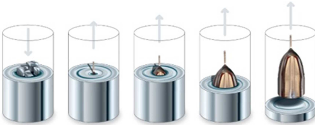
Figure 1. Feedstock is melted in a crucible. A seed introduced to the surface induces crystallization. As the seed is rotated, it is slowly drawn upward resulting in a boule.
