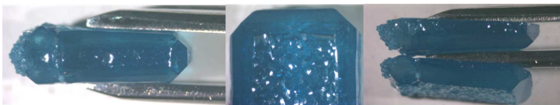
Figure 28. An as-grown Yb:LuAG on YAG crystal shows attached SN (left) on one end of the blue crystal and normal hillock growth (center). Two slabs result from cutting through the YAG seed lengthwise which will then be polished away.
