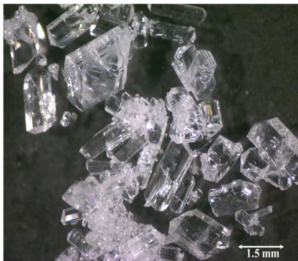
Figure 45. Hydrothermal treatment of components with hydroxides leads to large well-formed crystals of dellaite \text{Ca}_6\text{Si}_3\text{O}_{11}(\text{OH})_2 .
