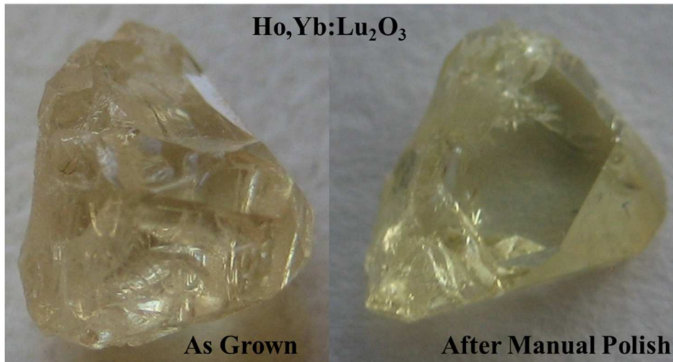
Figure 64. A small clear window was polished open for spectroscopy in this 0.45%Ho, 1.57% Yb:Lu 2 O 3 crystal with a final path length of 2.10 mm.
