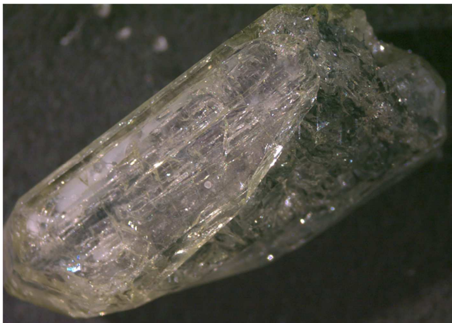
Figure 118. Out of control growth of TAG with blue internal growth covered by colorless growth.
