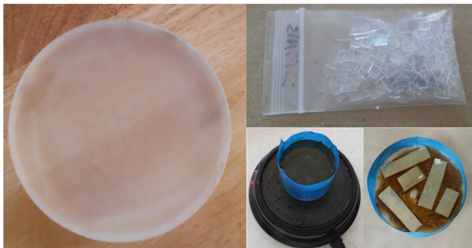
Figure 63. Flattened glass lap, left. Spacers, right top, and bottom, right, guard against rounding of the crystal.
