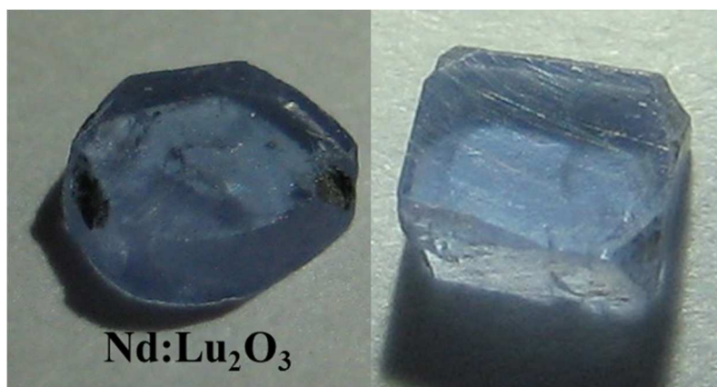
Figure 83. The Nd-doping percentage, estimated by EDX, is 1.2%. These crystals grown by SN are about 3.5 mm in length.
