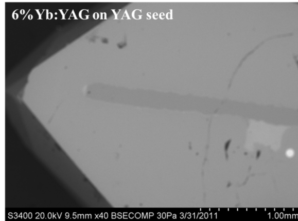
Figure 18. An SEM image looking end-on through a cross-section of Yb:YAG on a YAG seed.
