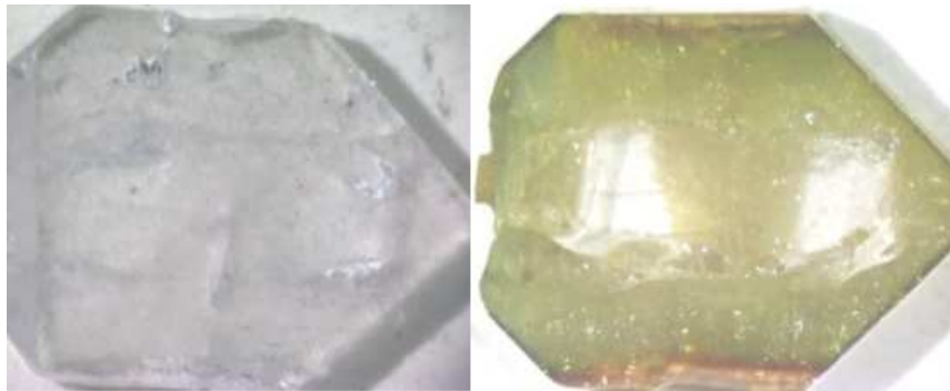
Figure 123. A co-doped YAG crystal grown from Ca/Cr:Y 2 O 3 plus Nd:Y 2 O 3 feedstock before annealing (left) and after (right). Absence of dark ring around the interface implies there has been a more homogeneous doping.
