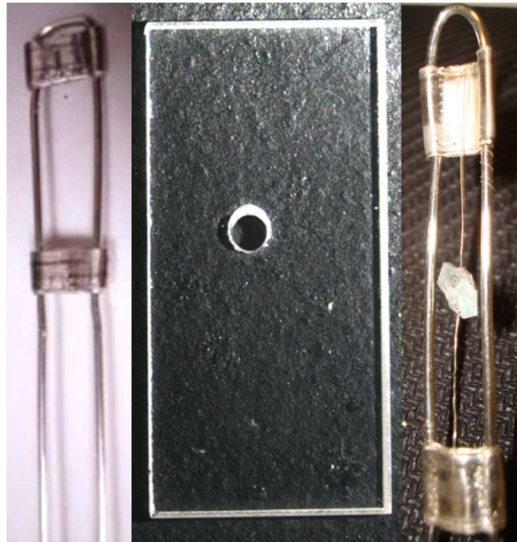
Figure 11. A silver ladder (left) holds a 1 – 2 cm YAG seed (center, magnified) in the growth zone, and a fully grown crystal still on ladder (right).
