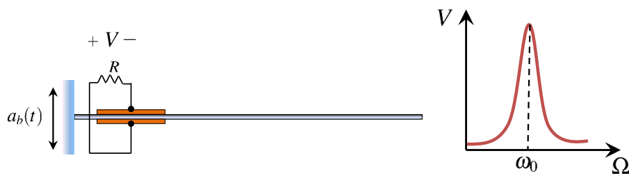
Figure 1.1: Schematic of a piezoelectric energy harvester.
