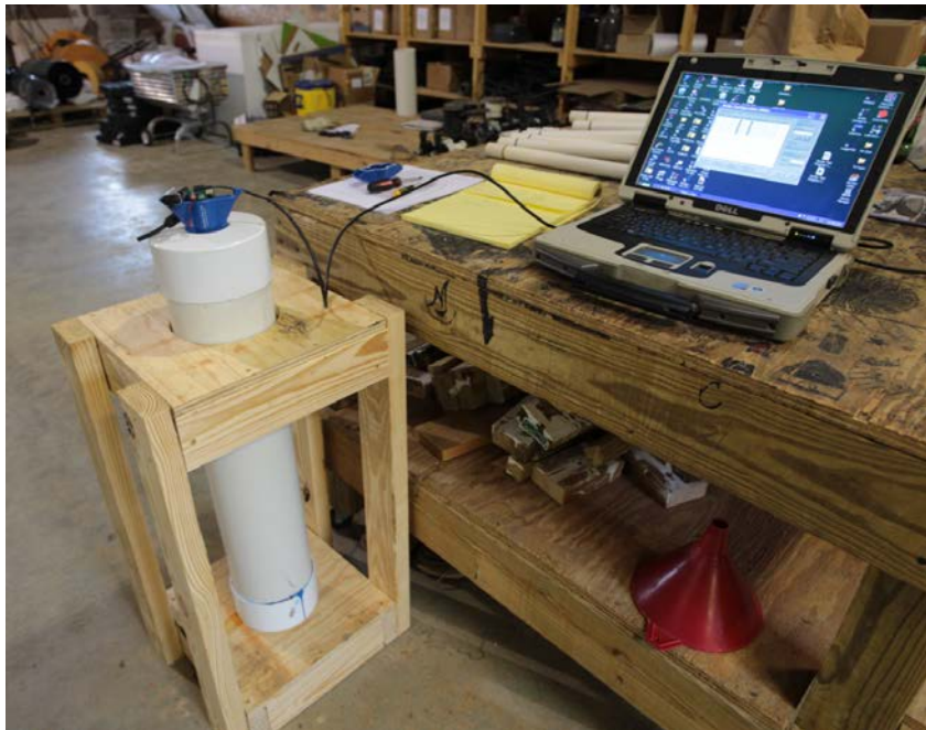
Figure 1.4 Normalization of Sentek EasyAg-50 probe in water.
