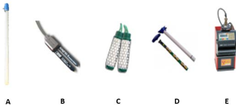
Figure 1.3 Soil moisture sensor used in this study were AquaSpy (A), Decagon EC-5 (B), Watermark 200SS (C), Sentek EasyAg50 (D), and 503DR Hydroprobe (E).
