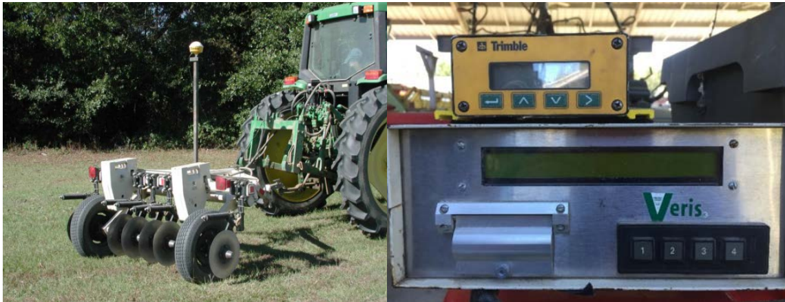
Figure 1.9 Veris 3100 EC meter (left) and Veris data logger accompanied with Trimble DGPS (right).
