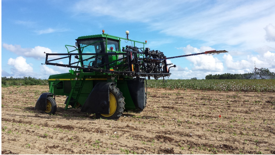
Figure 2.7 GPS antennas mounted on back of a high-boy sprayer during 2014 growing season
