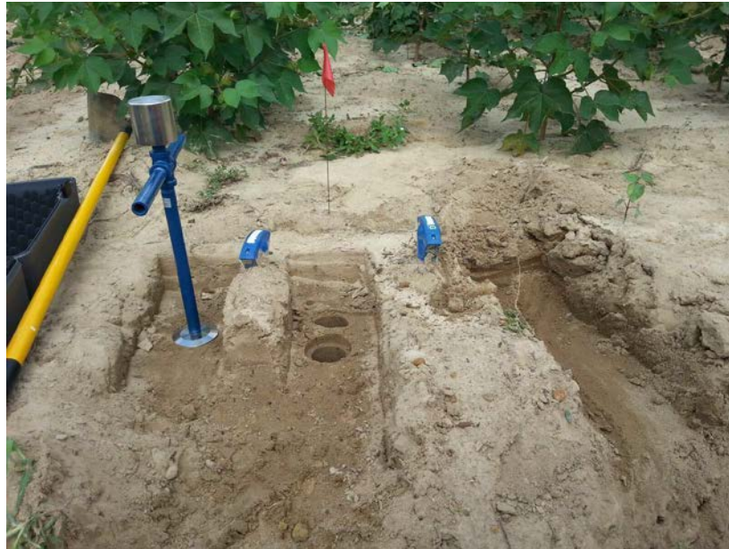
Figure 1.6 Taking soil samples near two Sentek EasyAg-50 probes.
