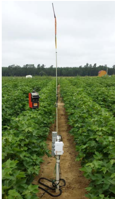
Figure 1.11 Decagon EC-5, Watermark 200SS data loggers, and 503DR Hydroprobe in the field in 2014 growing season.
