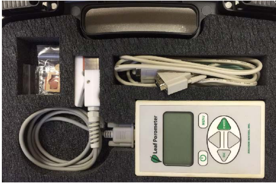
Figure 2.10 SC-1 Leaf Porometer
