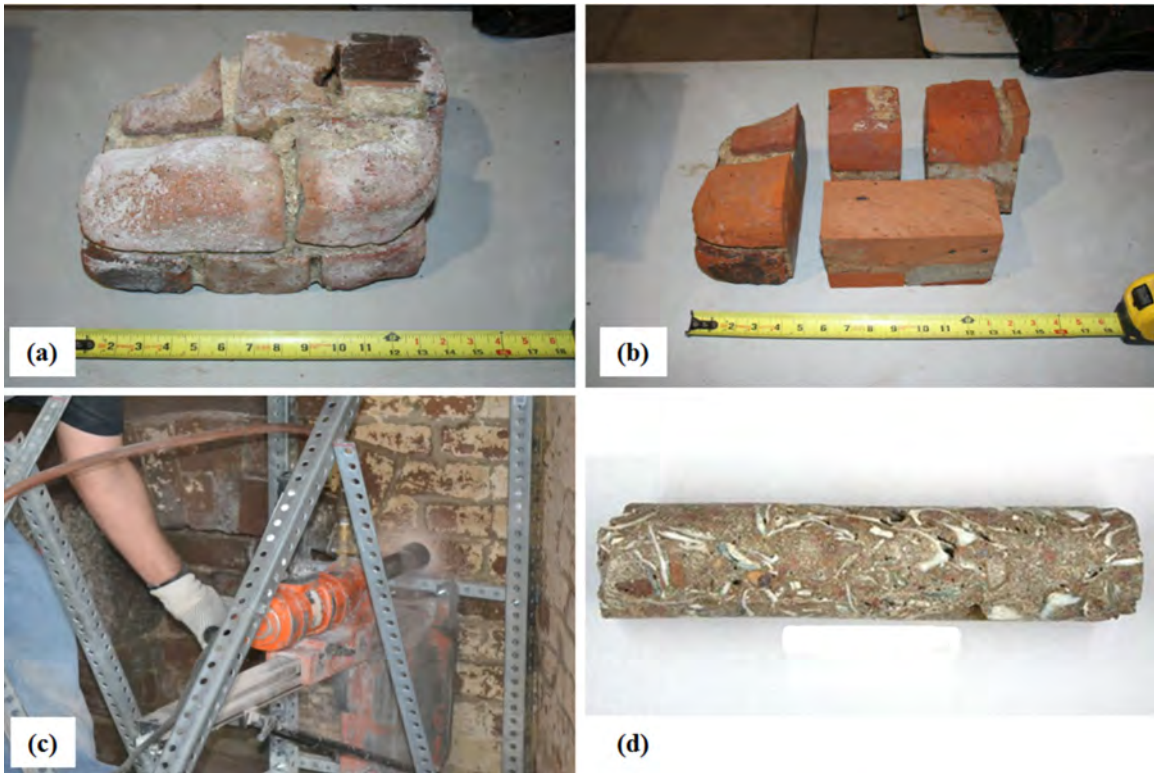
Figure 27: (a) Block specimen from the remains of the fort; (b) block specimen segmented into smaller samples for testing; (c) Coring of the wall in progress; (d) an intact core sample of tabby concrete infill.
