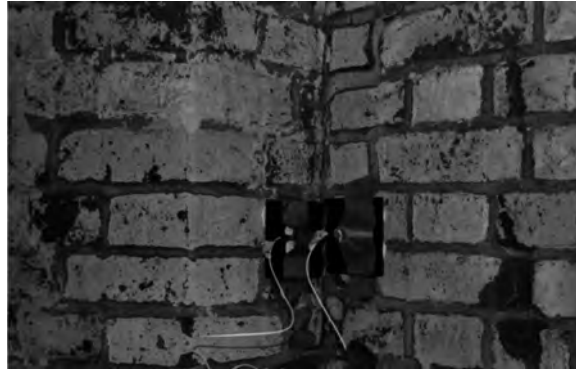
Figure 36: Test set-up on the North pier of Casemate 4 showing two adjacent accelerometers mounted parallel to the scarp wall interface with one accelerometer on the pier and one on the scarp wall.
