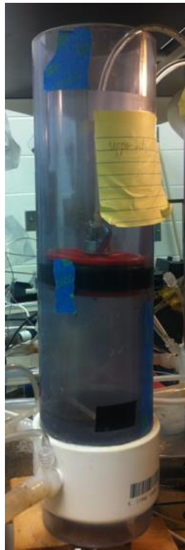
Figure 2.8: An air chamber in the system.
