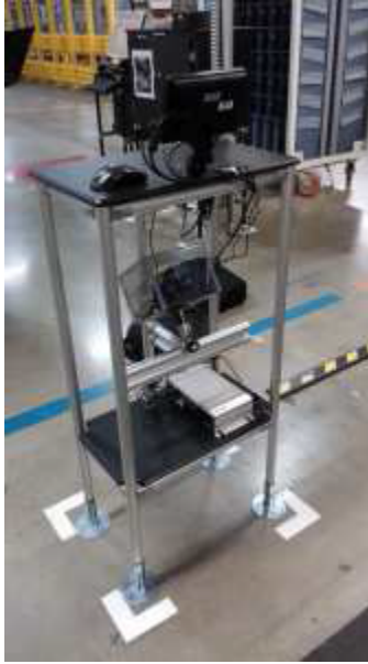
Figure 1.1: The VI system mounted on fixed stand which includes the computer, display and camera.
