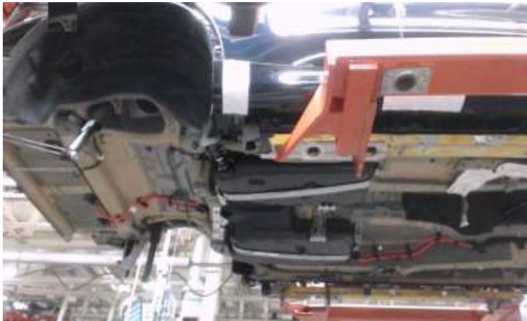
(b) Spring coil not installed.
