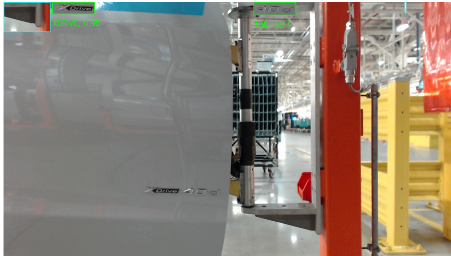
Figure 1.2: Screenshot of a successful inspection which is shown as output to the human inspector.
